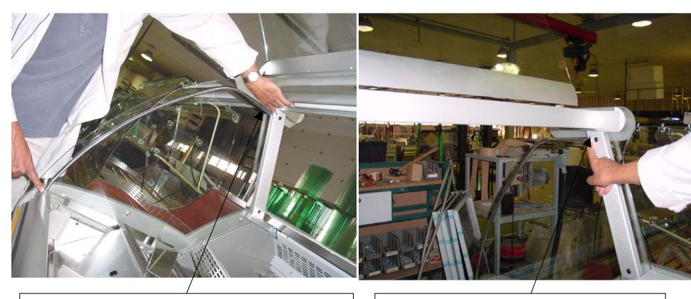
12) Place the tube that supports the structure in the front and upper gadgets as shown.
