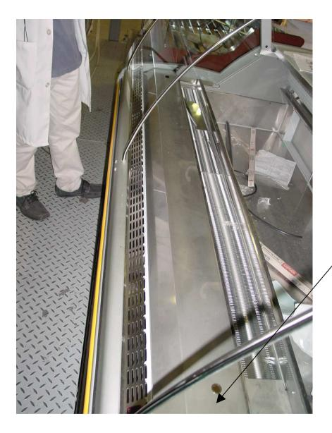
**8)** Place the metal sheet taht covers the ventilators
