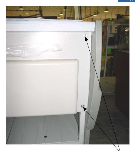
**4)** Screw with key « Umbrako » N°.5 to assemble these parts
